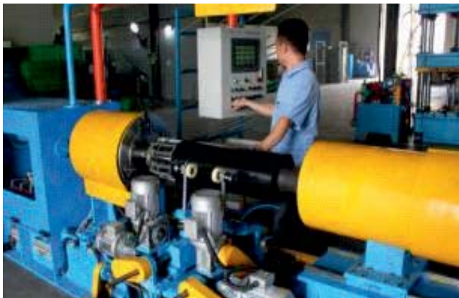
Maszyna do Formowania Gumy / Building for Rolling Lobe Type for Chassis Suspension
